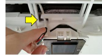
You will need to slide the filter out slightly to feed the connector through
