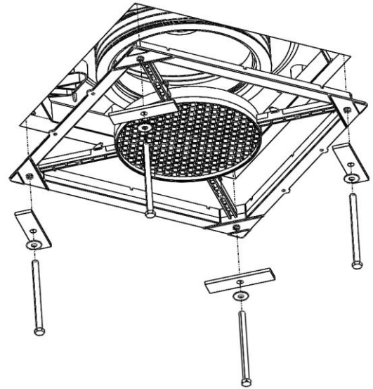
Figure 9- Assemble Bolt, washer & bar into duct & brace
