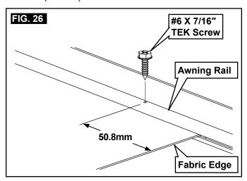
5. Pull to stretch opposite edge of awning fabric approximately 19.05mm. Then secure with #6 X 7/16" TEK screw through awning rail (approximately 50.8mm from fabric edge).
