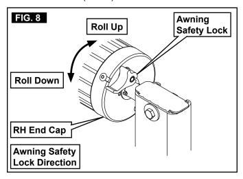
7. AWARNING IMPACT OR PINCH HAZARD. Do NOT remove nail from torsion rod (at end cap) until BOTH arm caps are secured to corresponding main arms, and awning safety lock lever is in roll down position. Otherwise, rapid casting spin off will occur. Spring tension will attempt to close the awning quickly and unexpectedly. Failure to obey this warning could result in death or serious injury.
