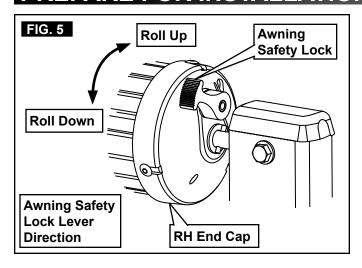
6. AWARNING IMPACT OR PINCH HAZARD. Do NOT remove cotter pin from torsion rod (at end cap) until BOTH top castings are secured to corresponding main arms, and awning safety lock lever is in roll down position. Otherwise, rapid casting spin off will occur. Spring tension will attempt to close the awning quickly and unexpectedly. Failure to obey this warning could result in death or serious injury.
