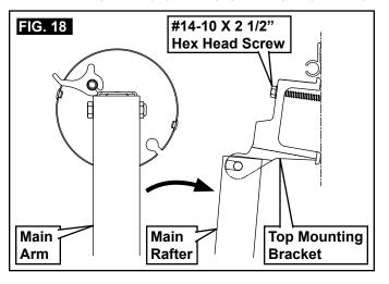
4. AWARNING FIRE OR ELECTRICAL SHOCK HAZARD. Make sure there are no obstacles (wires, pipes, etc.) inside RV's roof and / or walls. Shut OFF gas supply, disconnect 220-240 Vac power from RV, and disconnect positive (+) 12 Vdc terminal from supply battery BEFORE drilling or cutting into RV. Failure to obey these warnings could result in death or serious injury. Drill 4.76mm diameter holes through marked mounting hole locations and into solid structure of RV.
