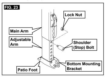
3. Pull lift handle out and slide main arm down until it rests on stop bolt. Then release lift handle to lock in position. See (FIG. 20) & (FIG. 23).
