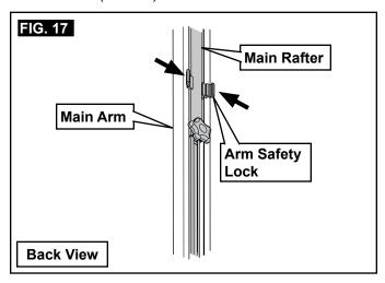
Make sure rafter is aligned directly behind and centered with main arm. Then carefully pull main rafter away from main arm (toward RV), and mark hole location for top mounting bracket. See (FIG. 10), (FIG. 11), (FIG. 12), & (FIG. 18).
