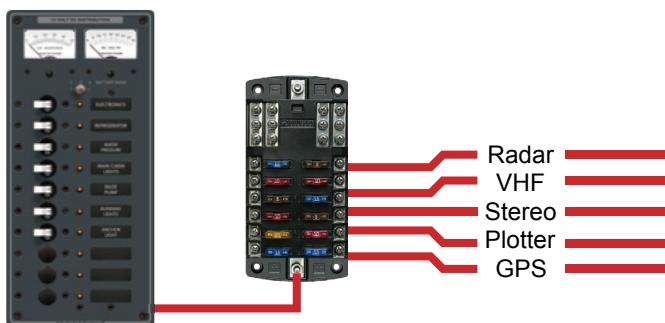
A 12 circuit DC circuit breaker panel costs 10 times more per circuit on average and takes up 3 times as much space. The example below illustrates this.
