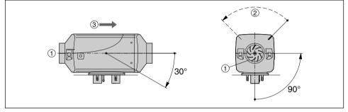
Heater air intake opening (fan wheel)
