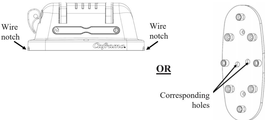
IV. Slide fan base onto firmly secured backing plate. Secure fan to backing plate with two screws provided.
