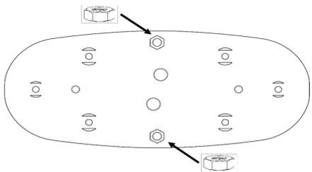
Place nuts in hex holes on back of backing plate before mounting
