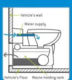
Fill central water tank via external water connection. Use Agua Rinse Spray in the toilet bowl before you flush the toilet.
