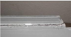
Destruction of a C1 window pane in the hinge area; Cause: Corrosive agent in detergent
