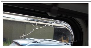
Cracks beginning from under the hinge profile of an S7 window;
