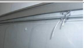
Large cracks in the hinge profile area – Outer pane already perforated, new cracks beginning to form on the surface, initially visible as spots;
