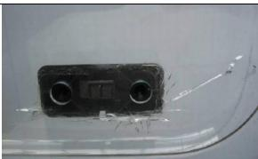
Cracks on the inner pane in the area of the anchorage of the catch;
