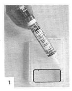
Apply a line of silicon caulking to the back side of the filter casing around the fan discharge opening
