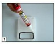
Apply a silicone beading on the rear of the filter housing around the fan outlet opening.
